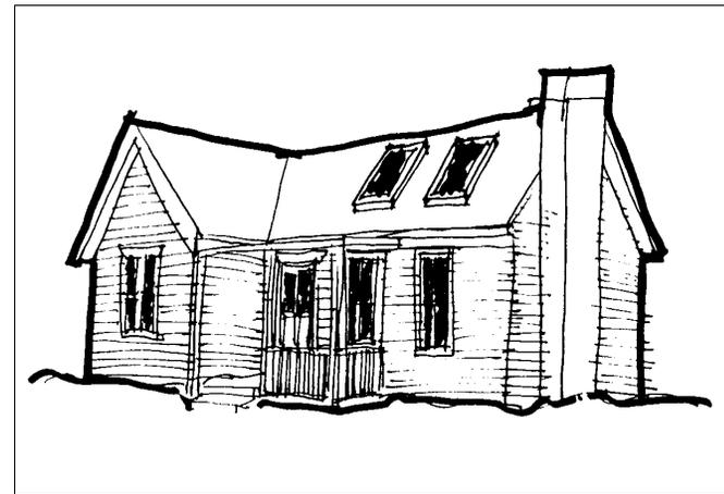
*Minimize the visual impact of solar collectors and skylights by placing them on roof slopes that are not visible from public ways*
