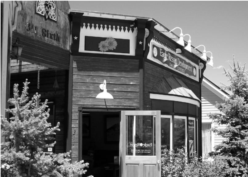
*Down-shielded lighting fixtures should completely cover the bulb from view.*
